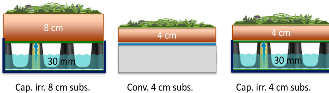
Figure 2. Schematic cross-sections of the three research plots. The left and right plot are equipped with the Permavoid drainage and capillary irrigation system.
